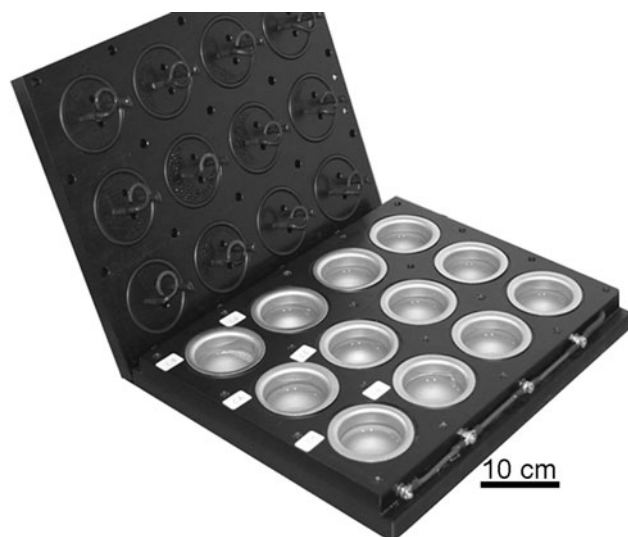
Fig. 1 Double biofilm analyzer (DBA) instrument with the lid open. The instrument consists of a platform with holders for 12 stainless steel vials of which six were individually polarizable. Each vial was provided with a wire electrode and a lid-mounted reference electrode so that they reached the vial when closing the lid. The vial operated as the counter electrode. The DBA instrument was operated in a rotating thermostatic incubator (45°C) that provided a liquid flow of 0.3 \text{ m s}^{-1} in each vial
